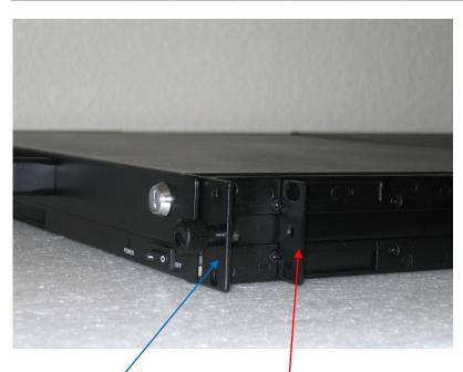
(1) First step: Unscrew the two thumbscrews on the front of
